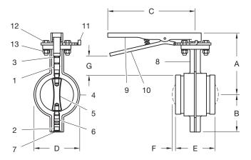
FIGURE 2 MODEL B303 BUTTERFLY VALVE WITH LEVER-LOCK OPERATORS
