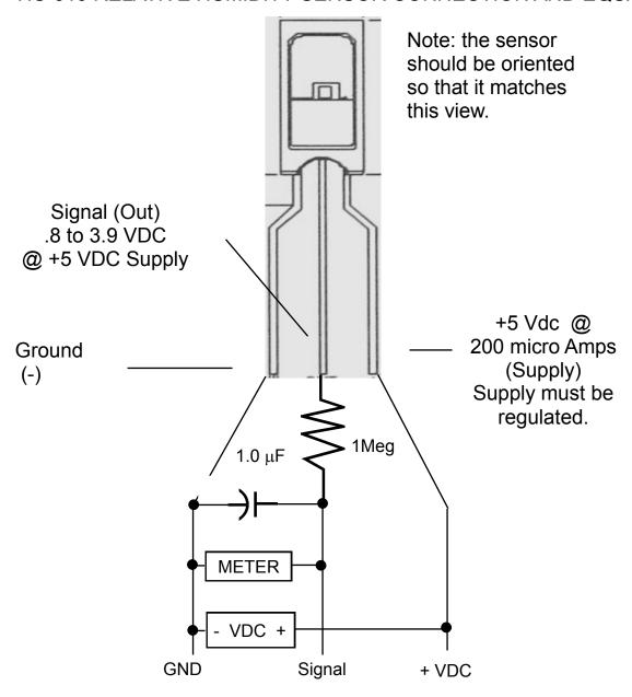
WARNING! Connecting the sensor wrong may damage the sensor. Double check your connections before applying power.
