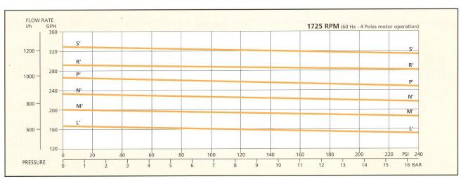
Characteristics at constant motor speed, with water at 68 °F and by-pass blocked - Figures of flow are averages - Pump weight: 1,9 kg (4,2 Lbs) clamp mount and 2 kg (4,4 Lbs) florage mount.
