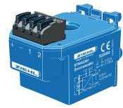
The STWA2AH is a measuring transducer for AC currents 0...100 A, divided in 2 ranges 0...20 A and 0...100 A. Multiple loops of the conductor through the transformer reduces the measuring range correspondingly (for instance to 0...5 A with four loops).
