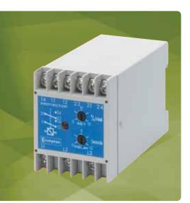
Three-phase, three or four-wire Adjustable set point Adjustable time delay Internal differential LED trip indication Double-pole relay contacts Automatic reset
