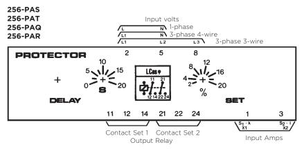
**Note:** Only one CT connection is required, from the same phase as the voltage connection to terminal 2.
