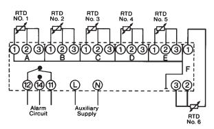
When used for less than 6 RTD inputs the unused terminals 1, 2 and 3 must be linked together.
