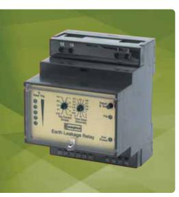
Precision digital settings LED bar graph display 10 selectable trip levels - 30mA to 10A 16 selectable time delay -0ms to 10 seconds Less than 40ms response time 0-1mA analogue output 8 amp 250V rated relay contacts User selectable energise or de-energise link Double-pole change over relay Single-pole pre-alarm option
