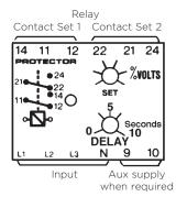
**Note:** The neutral connection is always used on four-wire systems.
