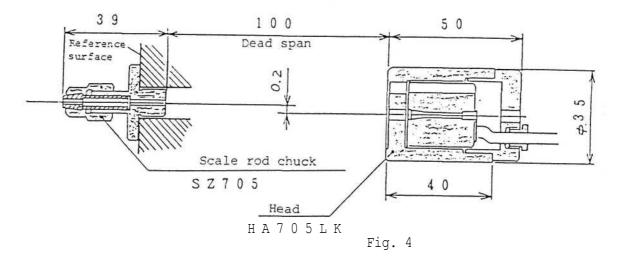
4-4). Fix the scale at the side where zero point is marked. Install the scale and the head parallel to the moving direction within their specified parallelism:
