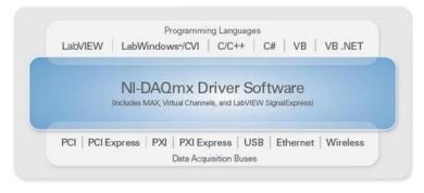
**Figure 4.** NI-DAQmx driver software abstracts data acquisition bus technology and provides a consistent API across multiple programming languages.
