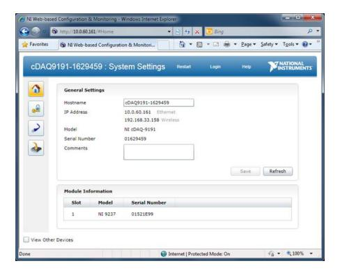
Figure 3. With the embedded Web server on the cDAQ-9191 chassis, you can remotely configure your NI CompactDAQ system from a Web browser.
