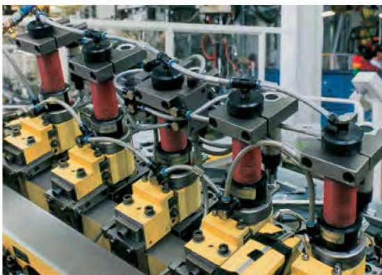
Stamping units placed in line
