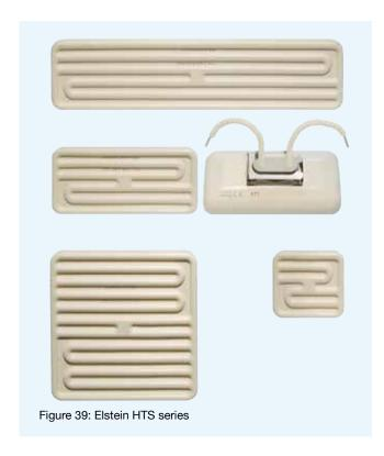
Elstein HTS high temperature heaters are ceramic infrared panel heaters, which can be used for operating temperatures up to 860 °C and surface ratings up to 64 kW/m².
