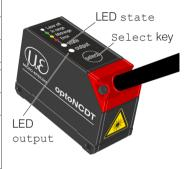
The programmable touch key select calls up the functions Masters and Teaching. By factory default this key is only active for the first 5 minutes after power up. After that it will be automatically locked. The keylock can be programmed via internal websites or ASCII commands.
