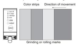
In case of rolled or polished metals that are moved past the sensor the sensor plane must be arranged in the direction of the rolling or grinding marks. The same arrangement must be used for color strips.
