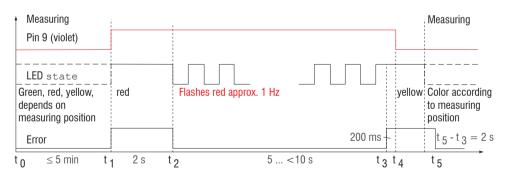
Fig. 43 Flow chart for the return of output scaling
