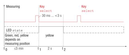
The function Zeroing/Mastering can be used several times in succession. Between repetition of the function Zeroing/Mastering a brake of 1 s is necessary. The function Zeroing/Mastering can also be combined with the multifunctional input.
