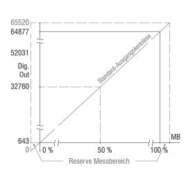
Fig. 37 Digital values without zero setting resp. mastering
