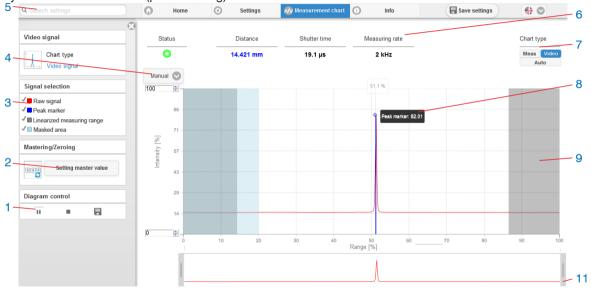
Fig. 28 Display of video signals
