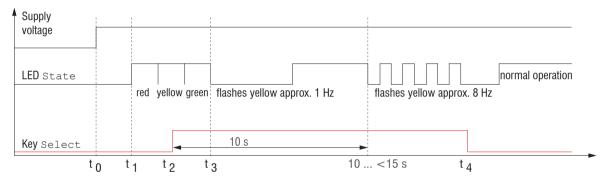
Fig. 50 Flow chart to start a sensor with factory setting
