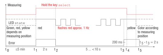
Fig. 41 Flow chart for the return of output scaling
