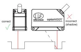
In case of bore holes, blind holes and edges in the surface of moving targets the sensor must be arranged in such a way that the edges do not obscure the laser spot.
