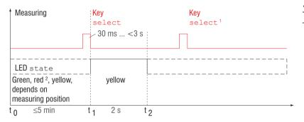
The key Select is locked according to factory settings after expiry of 5 min. You can unlock the keylock e.g. via the web interface, see Chap. 7.6.3.
