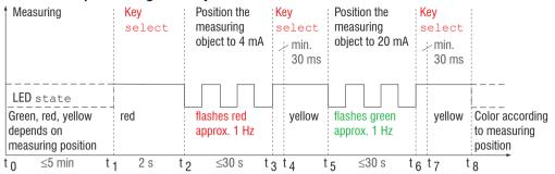
Fig. 40 Flow chart for output scaling
