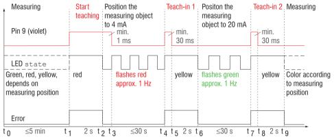
Fig. 42 Flow chart for output scaling
