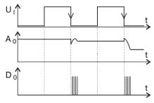
Fig. 31 Trigger edge HL (above) with analog output A and digital output signal D (below)
