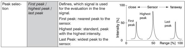
A correct measuring result can be determined only for the first peak when a measuring object which consists of several transparent layers.
