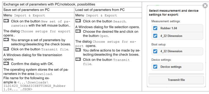
A security query, see adjacent figure, helps to avoid that an existing setup is inadvertently overwritten during import.
