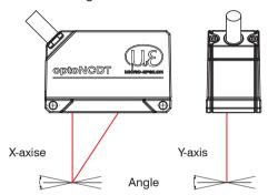
Fig. 9 Measurement errors through tilting with diffuse reflection
