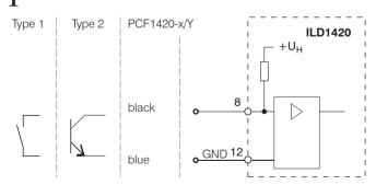
There is no external resistor for current limiting required. Connect Pin 8 with Pin 12 for permanent "Laser on".
