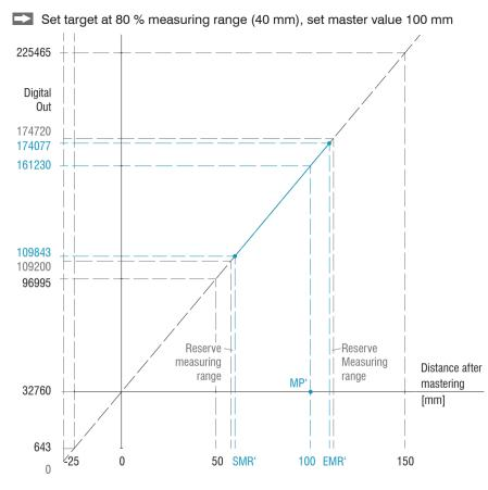
Fig. 38 Digital values of an ILD1420-50 with mastering, master value 100 mm
