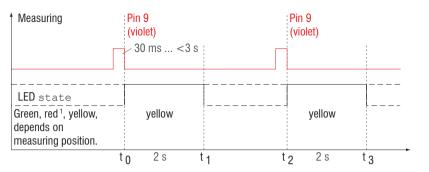
Fig. 35 Flow chart for zeroing, mastering (hardware input)
