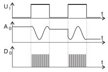
Fig. 30 High trigger level (above) with analog output A and digital output signal D (below)
