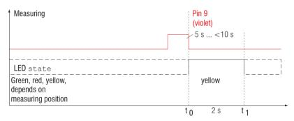
Fig. 36 Flow chart for the return of zero setting and mastering
