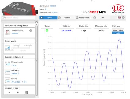
In the top navigation bar other auxiliary functions (settings, measurement chart etc.) are available.
