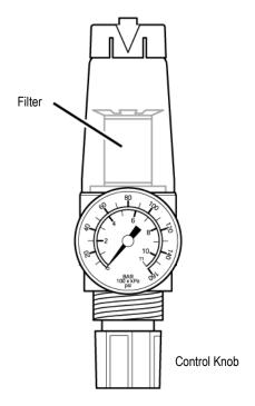
Figure 82: Air Purging Flow Regulator with air filter (E-AR)
