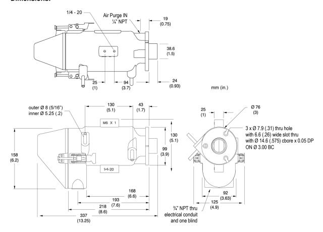
Figure 68: Dimensions for the ThermoJacket
