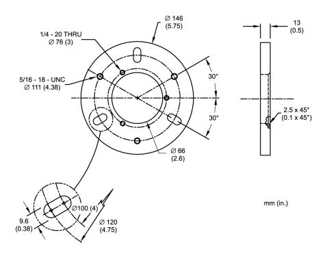
Figure 69: Mounting Flange for ThermoJacket (E-MF)
