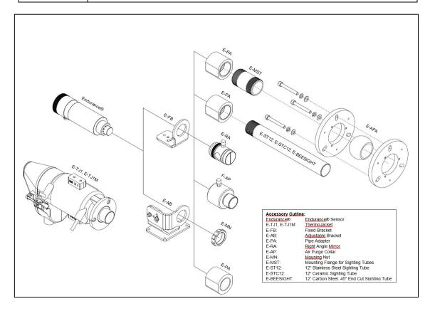
Figure 52: Extraction view of Endurance® sensor with mechanical accessories
