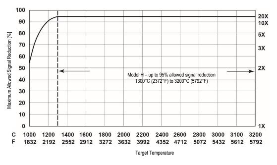
Figure 85: Model H Percentage of Allowed Signal Reduction
