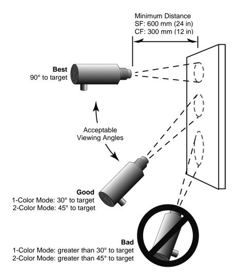
Figure 7: Acceptable Sensor Viewing Angles
