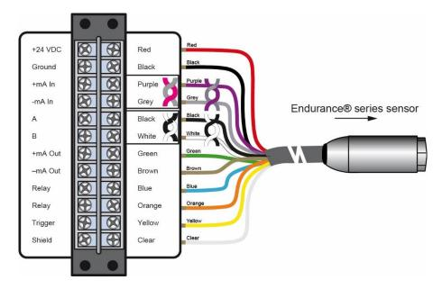
Figure 15: Endurance® series labeled terminal block
