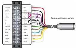
Figure 45: Endurance® Terminal Block in a NEMA 4 Enclosure (E-TBN4)
