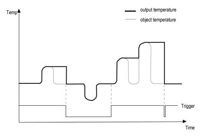
Figure 30: Peak Hold reset by external Trigger signal
