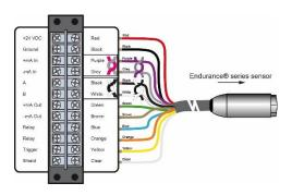
Figure 44: Endurance® Terminal Block (E-TB) with wire color assignment
