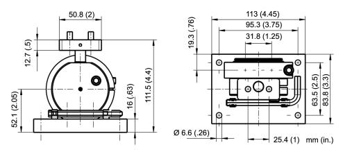
Figure 70: Adjustable Mounting Base for ThermoJacket (E-MB)
