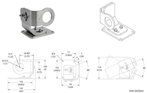
Figure 57: Adjustable bracket (E-AB)
