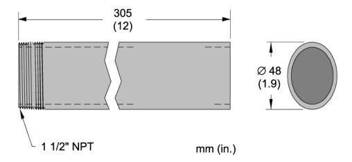
Figure 76: Ceramic Sighting Tube (E-STC12)
