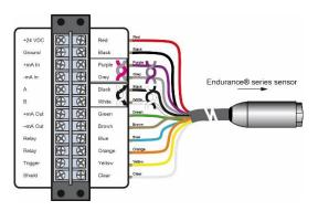
Figure 40: High Temp. Multi-Conductor Cable with M16 Connector (E-2CCBxx)
