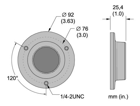
Figure 75: Mounting Flange for Sighting Tube (E-MST)
