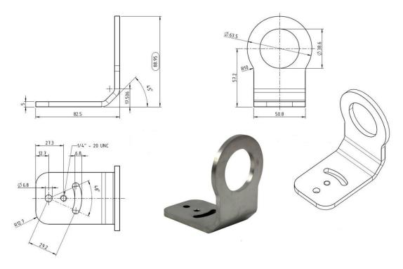
Figure 56: Drawing and Photo of Fixed Bracket (E-FB)
