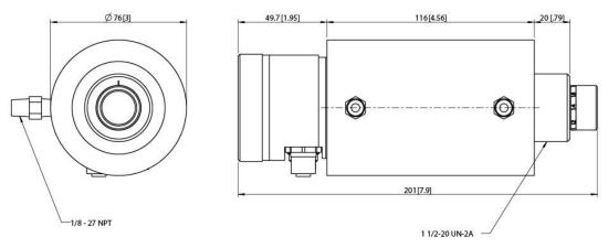
Figure 4: Dimensions of Endurance® Sensor in Air/Water-Cooled Housing Option
