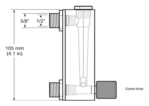
Figure 81: Water Flow Regulator (E-WR)
