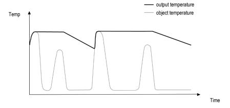
Figure 32: Linear Signal Drop (decay mode)
