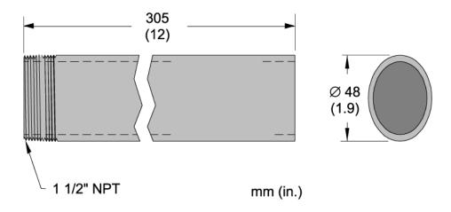
Figure 77: Stainlless Steel Sighting Tube (E-ST12)
