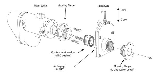
Figure 73: Mounting the Blast Gate Assembly
