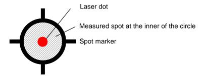
Figure 37: LASER Spot Size Indication
