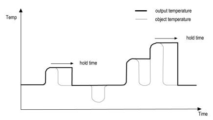
Figure 29: Peak Hold reset by Peak Hold Time expiration
