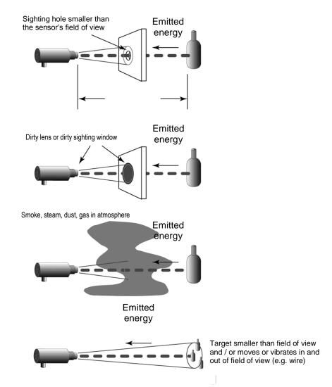
Figure 6: Sensor Placement in 2-Color Mode
