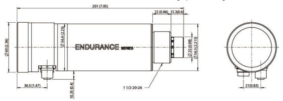
Figure 3: Dimensions of Endurance® Sensor
