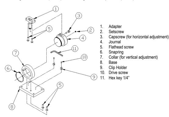
Figure 71: Explosion view of the Adjustable Mounting Base (E-MB)
