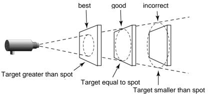
Figure 5: Proper Sensor Placement in 1-Color Mode
