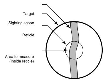
Figure 8: Sensor Eyepiece and Reticle
