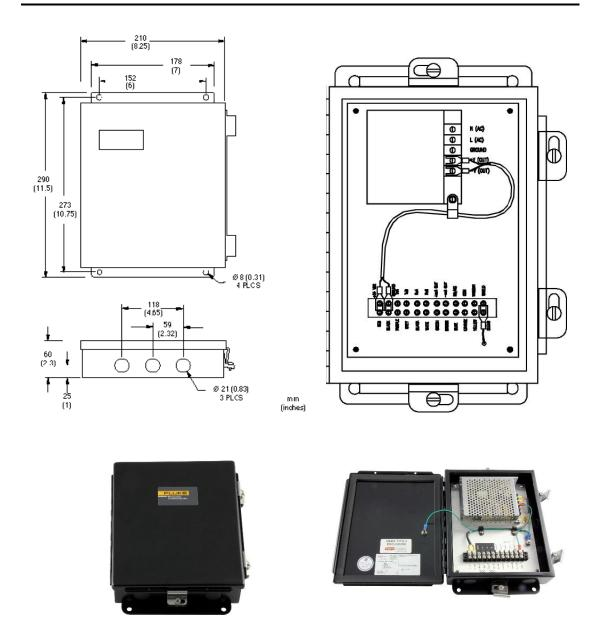
Figure 47: 24VDC, 1.1A, 100-240VAC power supply in NEMA 4/IP65 case (E-PS)
