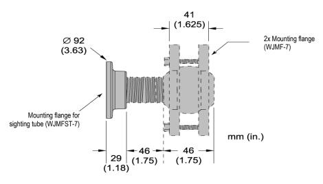
Figure 74: Adjustable Pipe Adapter (E-APA)
