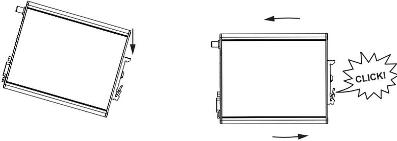
The MRD-315 includes integrated mounting flanges and can be attached to a panel or tray by means of screws, using the slots provided. Alternatively the MRD-315 can be DIN rail mounted, using the DIN rail mounting kit.
