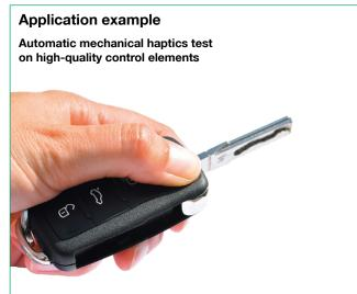
Inspecting the tactile behavior entails the precise measurement of the most minute operational forces, click ratio, blocking loads, et al.
