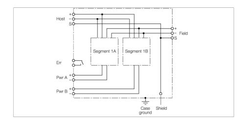
The DPC system (Diagnostic Power Conditioner) is a power supply system for the installation of FOUNDATION  $^{\text{TM}}$  fieldbus H1 segments.
