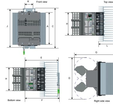
The diagram below shows a 125A EPackLite (doors open), 80 and 100A units are similar- refer to Table 3 for dimensions. Table 3 Dimensions for EPackLites of different current ratings (all values in millimetres)
