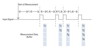
Figure 1. Buffered Period Measurement with Counter/Timers
