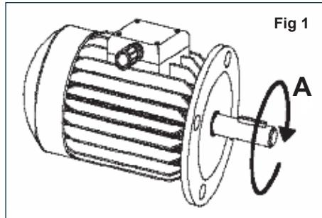
Before acting on the terminal board or electrical connections, make sure the plant is disconnected from the electric power supply. The terminal board is closed with a black polycarbonate or metal lid. The wire connection terminals are made of brass and all internal connections are made in conformity with standard IEC34-8.
