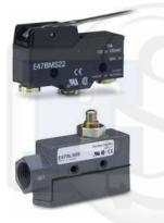
Precision switches are typically available in two types: basic precision and enclosed precision. The basic precision switch is of onepiece construction. The enclosed precision switch is simply a basic switch inside a die cast housing. Basic precision switches are generally not given a NEMA enclosure rating, while some enclosed precision switches can be rated NEMA 4 or 13.
