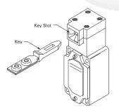
Actuation of the interlock switch occurs only when the corresponding key is inserted into the key slot. The key is usually mounted on a door or machine guard in such a way that when the door or the guard is closed, the key fits into the slot actuating the switch. The special key design makes the safety interlock switch extremely difficult to defeat. When inserted into the slot, the key performs three separate mechanical functions.
