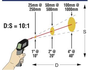
The MiniTemp MT6 thermometer is intended for close range targets, measuring a minimum target area of 1 inch in diameter from a distance of approximately 10 inches, and measuring approximately a 6 inch area from 5 feet away.
