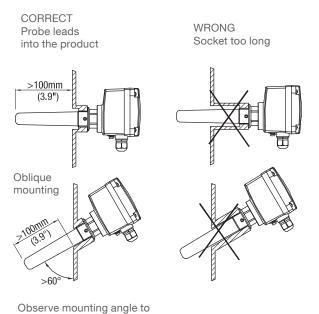
Observe min. distance between two sensors, to metal silo wall and to protective angle.
