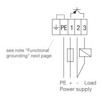
Approved power supply with reinforced insulation to mains is required
