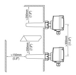
ensure, that the active tip of the probe has enough distance to the metal silo wall
