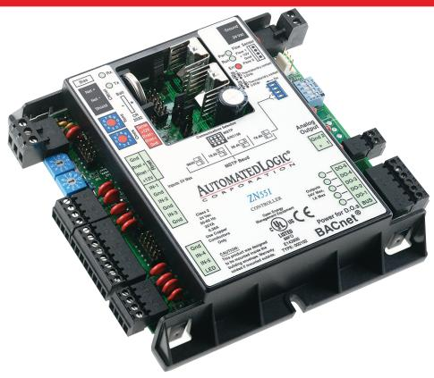
Automated Logic's ZN551 provides unprecedented power and flexibility through fully programmable networked controllers. The ZN551 controllers connect to the Building Automation System (BAS) network using BACnet over ARCNET 156 Kbps or MS/TP. The ZN551 supports a line of RS room sensors using Rnet port.
