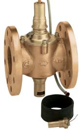
541 tech. broch. 01046 Fuel shut-off valve for high pressure use. Bronze body. Flanged connections PN 16. To be coupled with flat counterflanges EN 1092-1. Max. working pressure: 50 kPa. Capillary length: 5 or 10 m. Settings: 98°C, 110°C, 120°C, 140°C, 160°C, 180°C.
