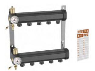
Max. working pressure: 6 bar. Max. hydraulic test pressure: 10 bar. Temperature range: -10–60°C. Ambient temperature range: -20-60°C. Medium: water, glycol solutions, saline solutions. Max. percentage of glycol: 50%. Manifold DN 50.
