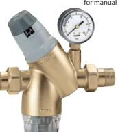
Stainless steel strainer cartridge with transparent housing. Male union connections. Max. upstream pressure: 25 bar. Downstream setting pressure range: 1–6 bar. Max. working temperature: 40°C. Strainer mesh size Ø: 0,28 mm. Certified to EN 1567. With replacement strainer and key to service strainer and cartridge.
