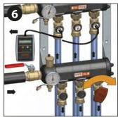
During the flow rate mesurement, the sensor creates no significant head losses and therefore causes no significant changes in the actual flow rate.
