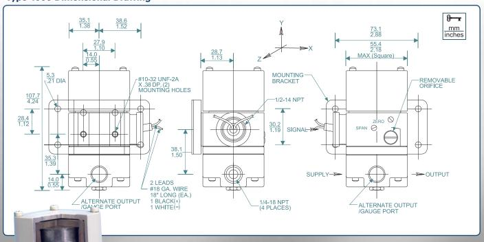
The Type 1000 has long been a standard in the I/P & E/P industry. With a built-in booster, the T-1000 provides
