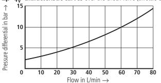
$\Delta \pmb{p} - \pmb{q}_{V} - \textbf{characteristic curves}$  over the check valve (throttle closed)
