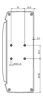
Note: Observe minimum spacing of >10 mm between the MEM's!
