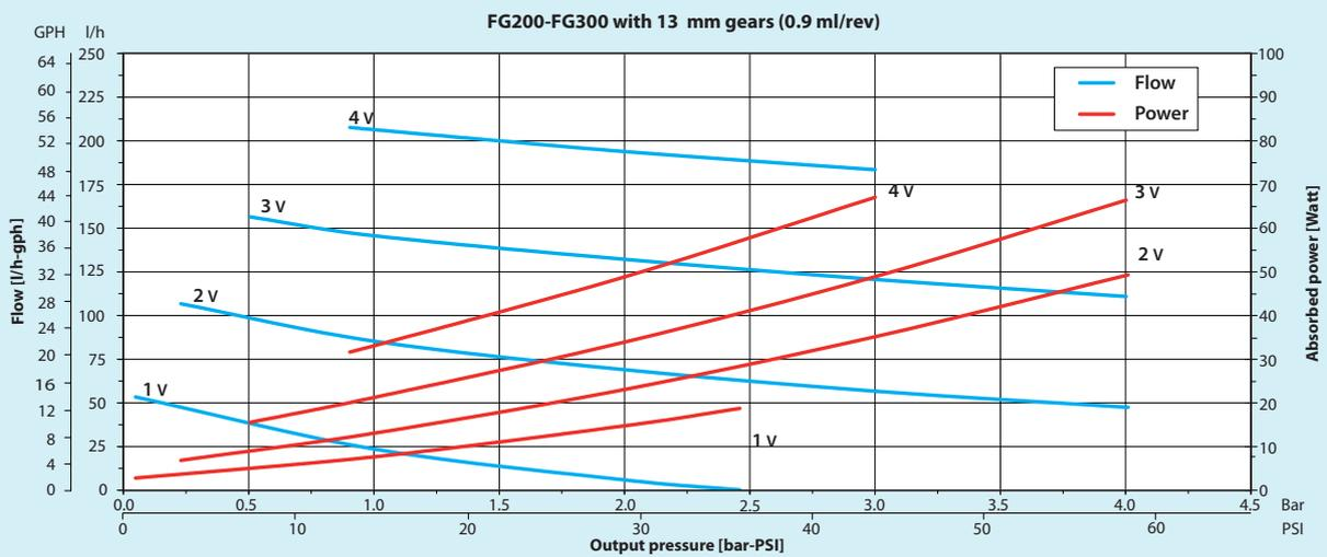
Note: Characteristics with water at 20 °C (68 F) and without relief valve. Use a filter before the pump inlet no larger than 10 micron. Temperature requirements different from ambient temperature must be mentioned on the order. Different materials are available upon request.
