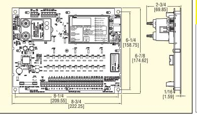
Simplify your on-demand cleaning requirements with the Series DCT1000DC Dust Collector Timer Controller. Relying on one timer board for on demand and continuous cleaning applications, the DCT1000DC eliminates external devices such as pressure switches, relays and timers.
