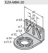
Mounting bracket, steel, blackfinished, for EZ-ARRAY and EZ-SCREEN standard 14 & 30 mm
