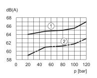
Approximate maximum values of noise level to minimum and maximum flow rate measured with the sound-level meter placed at one meter from pump coupling with flexible coupling.
