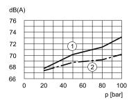
Approximate maximum values of noise level to minimum and maximum flow rate measured with the sound-level meter placed at one meter from pump coupling with flexible coupling.
