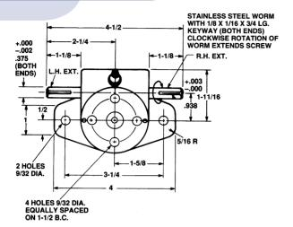
1/2" Diameter x .250 Lead Lifting Screws
