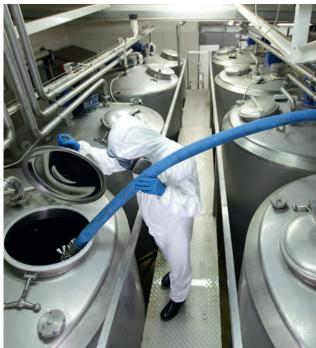
In applications with specific hygiene standards or in lines with aggressive (i.e. gaseous, chemicals, pharmaceuticals or varnish products) liquids, premium quick connect coupling systems are required. These systems allow a safe and reliable process within the connected system machinery or tool.
