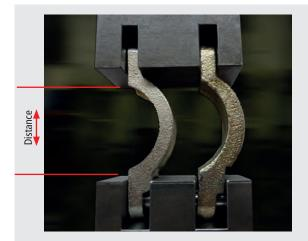
To illustrate the differences between the material qualities, **LUDECKE** consequently conducts fracture test with two hose clamps (original Luedecke hose clamp vs. a counterfeit from Far East) were inserted into a hydraulic press and tested under pressure.
