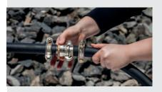
To ensure a proper locking, the MODY safety screw type coupling is locked with an additional locking nut underneath the claw head.
