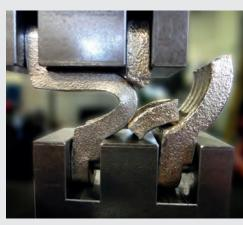
Distance of 23 mm (completely destroyed counterfeit, no cracks in the *LUDECKE* hose clamp)
