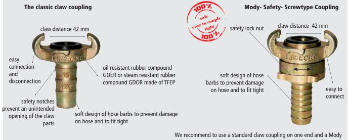
We recommend to use a standard claw coupling on one end and a Mody Safety version on the other end. This connection is absolutely safe, easy to couple and 100 % sealed.
