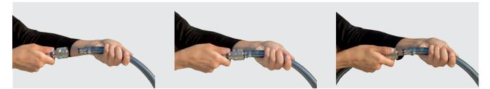
To disconnect, grasp the plug firmly with one-hand. With the other one push the locking sleeve backwards and pull the plug off the coupling. After disconnecting, the locking sleeve slips automatically back to starting position. This system allows not only a fast work process, but also a reduction to a minimum of potential injuries in term of finger trapping etc.
