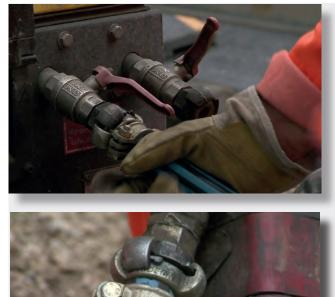
The **LUDECKE** success story started with the development of claw couplers. To date, this coupling type is used worldwide in various compressed air applications in the industrial and construction industry.
