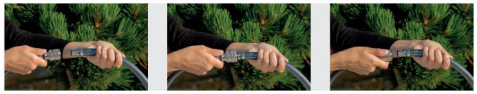
To disconnect, grasp the plug firmly with one hand. With the other hand push the locking sleeve backwards and pull the plug off the coupling. After disconnecting, the locking sleeve slips automatically back to starting position. This system allows not only a fast work process, but also a reduction to a minimum of potential injuries in term of finger trapping etc.
