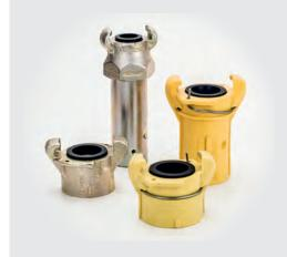
In applications such as sandblasting cabins or machines the use of **LUDECKE** sandblast couplings and nozzles is essential in order to provide best results. This system is related to the claw coupling design, but different in dimensions with a 58 mm claw distance. All dimensions are identical on the front side and interchangeable with each other regardless of the connection port dimensions.
