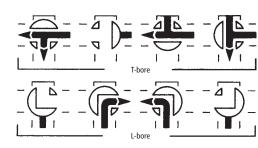
Flow direction diagram of T- and L-bore.
