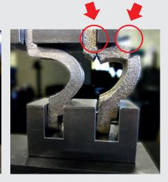
Distance of 28 mm (complete break in the counterfeit, no rupture in the *LUDECKE* hose clamp)
