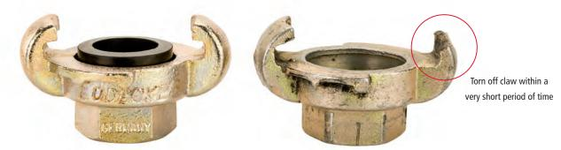
Original LUDECKE Claw Coupling (DIN 3489) Counterfeit from the Far East (no manufacturer's branding, inferior material)
