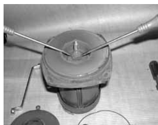
1) Detach the shaft seal using two screwdrivers. Do not damage the sealing surface of the shaft.
