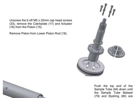
Remove the Sample Tube Balseal (79) and Slydring (80) from the Sample Tube.
