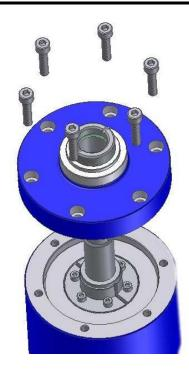
Apply slight air pressure to Port B in the Bottom Housing (13), and withdraw the complete sub-assembly comprising Piston/Catchplate/Sample Tube Actuator/Lower Piston Rod/Sample Tube/Capture Tube.
