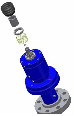
Remove the Gaiter (36) to expose the machined flats on the Sample Tube Actuator (16) through the Spring (30).
