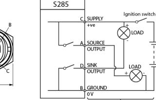
NOTE: IF SINK ONLY OUTPUT IS REQUIRED THEN PIN A IS NOT USED.
