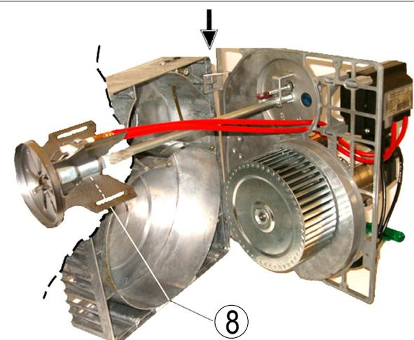
The plate must be fastened as indicated in the figure. By loosening the screw -8 you can pull out the flame disc.
