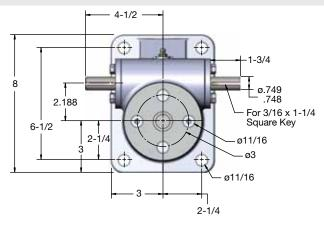
1-1/2"Diameter x .375 Lead Lifting Screws
