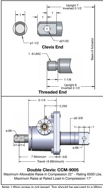
Note: Lifting screw is not keyed. Top should be secured to a lifting member to prevent rotation. When a Bellows Boot is required, see pages 148-149. Dimensions are subject to change without notice.
