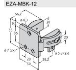
3071756 Mounting bracket, steel, blackfinished, for EZ-ARRAY and EZ-SCREEN standard and cascade 14 & 30 mm
