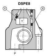
X: M6x8 plug for external pilot Y: M6x8 plug for external drain
