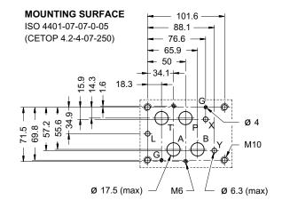
Single valve fastening: N. 4 TCEI M10x60 bolts - ISO 4762 N. 2 TCEI M6x60 bolts - ISO 4762
