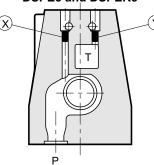
X: M5x6 plug for external pilot Y: M5x6 plug for external drain
