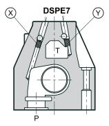
X: M6x8 plug for external pilot Y: M6x8 plug for external drain
