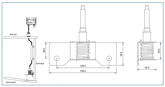
The brackets are U-shaped and manufactured of 2 mm ASTM 316L plated steel. Diameter of mounting holes: 11.5 mm. The transducer is secured by means of a spring fitted into two holes in the "U" shape, and can be mounted/dismounted without the use of tools.
