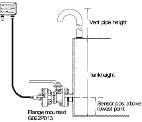
To ensure measuring accuracy a transducer type within the range no. 4, 5, 6, 7 and 8 is recommended.
