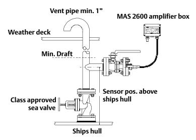
Transducer measuring range > max. draft minus sensor position.
