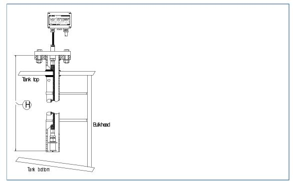
A top flange made of ASTM 316L connected to a Stainless Steel braided PTFE tube by fittings fixed to the tube by using special tools. A fitting in the opposite tube end is fixed to the transducer by means of nut and ferrules. Minimum hose bending radius is 130 mm.
