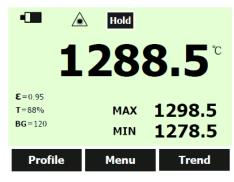
Press <Profile> to enter the first level menu selection. Each displayed name is edited under the PC interface, and then uploads to the instrument. Here the user can continue to the next screen using the arrow keys if the item quantity is more than 15.
