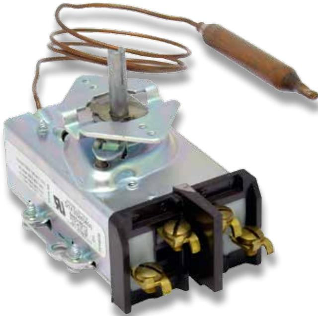
The Robertshaw® D1/D18 series is a heavy duty thermostat designed for use in harsh applications where precise temperature control is required. The control uses a double pole single throw (DPST) snap action mechanism with a positive OFF switch. It is recommended for use on applications that require double pole operation and accurate temperature control.
