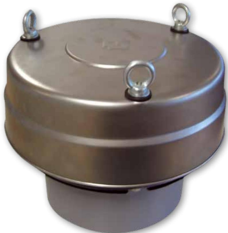
VCP Pressure Relief Valves consist of a cylindrical casing with clamped weld-on spigot, a disc shape inner steel lid for negative pressure operation held in position by a central spring rod, an outside steel ring for excess pressure kept in position by three spring rods, gaskets, and a weather protection cover.
