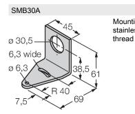
3032723 Mounting bracket, rectangular, stainless steel, for sensors with 30mm
